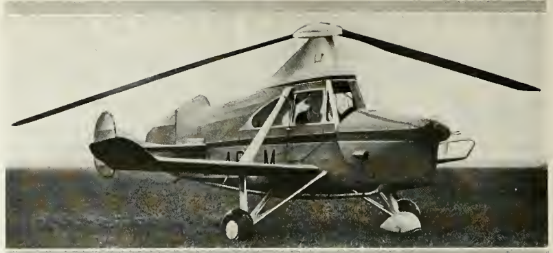
The new cabin autogiro built in England. It has three rotor blades
